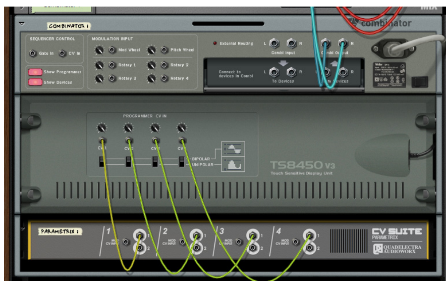
Fig. 4.1-1: CV Suite Parametrix, set up to control a Combinator's additional CV Inputs as parameters.
